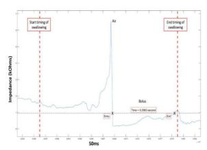
**Figure 3:** Impedance change measured during the bolus transmit over a single impedance channel. A rapid increase in the impedance channel is noted when the air through the impedance segment. The drop in the impedance channel is the higher conductive bolus material passes through the measuring site. The criteria is fulfilled the bolus successfully transmit through the region which the impedance located in the transition zone of esophagus.
