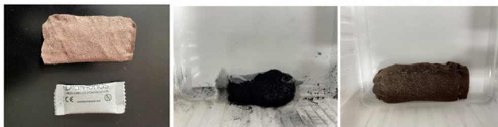
Figure 1: potential of absorption with super-absorbers: (a) below superabsorber sachet or bag and above sewn-in pack; (b) fragile sachet bursts after excessive fluid absorption; (c) sewn-in superabsorber-pack with sachet after absorption still intact.
