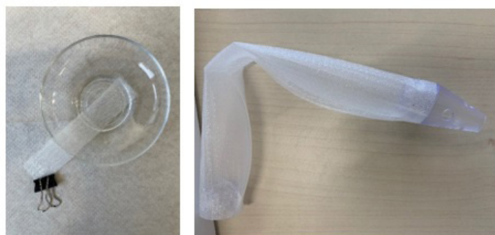
Figure 3: test for capillary effect from a water-basin without suction over a height of 1,0cm:
